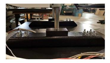
6. Remove the (16) nylon hex nuts that attach the black mounting tubes to the heater block assembly. Then lift the handle to cause the tubes to lift up and over the threaded studs that come out of the heater block assembly. At this point, the heater block is detached completely mechanically as well as electrically.
